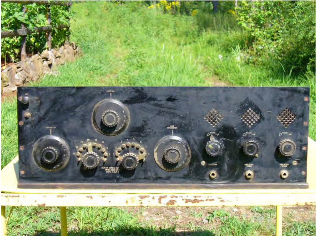
Doron Bros. Electric Company c1920 "Type R.D.2-A" 3-tube battery radio
